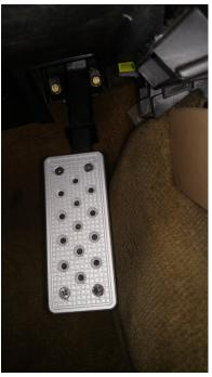
6) Put the throttle pedal cover into position and attach using the supplied self tapping screws. The throttle pedal is made of plastic so be careful not to over-tighten the screws.
