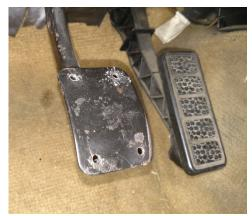
4) Mount the brake and clutch using the supplied stainless machine screws and lock nuts. Use the supplied 3/32" Allen key and a 9mm wrench to tighten the fasteners in position.
