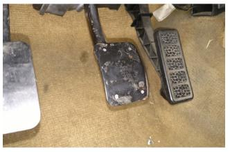
3) Using the pen marks made earlier as a guide, use the center punch to mark the holes on the brake and clutch pedals. The center punch marks will make it easier to start the holes with the drill and will ensure that the drill holes start in the correct locations. Use the 1/16" drill bit to drill pilot holes, followed by the 3/16" bit.
