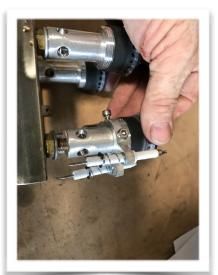
Next align needle so the two spikes are facing out to install the wires onto needle:
