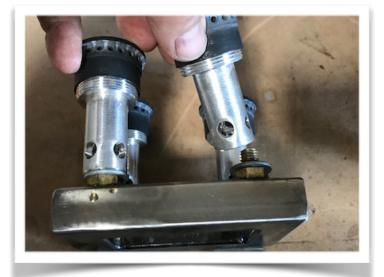
Burner heads and stems unscrew from burner base:
