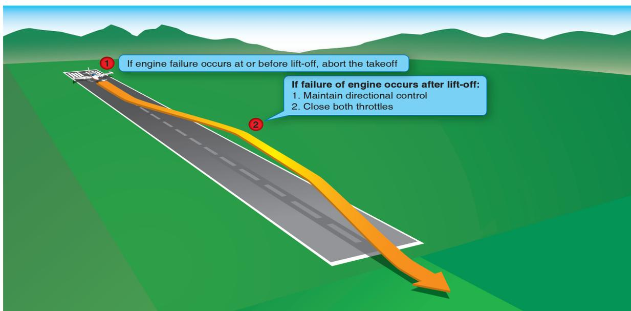
Figure 13-18. Engine failure on takeoff, landing gear down.
