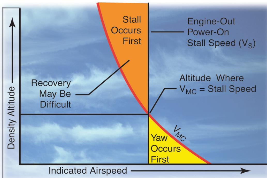
Figure 13-14. Graph depicting relationship of  $V_{MC}$  to  $V_S$ .
