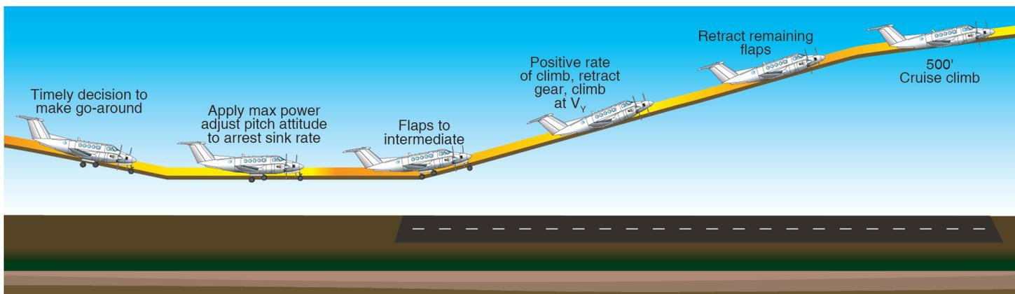
Figure 13-11. Go-around procedure.
