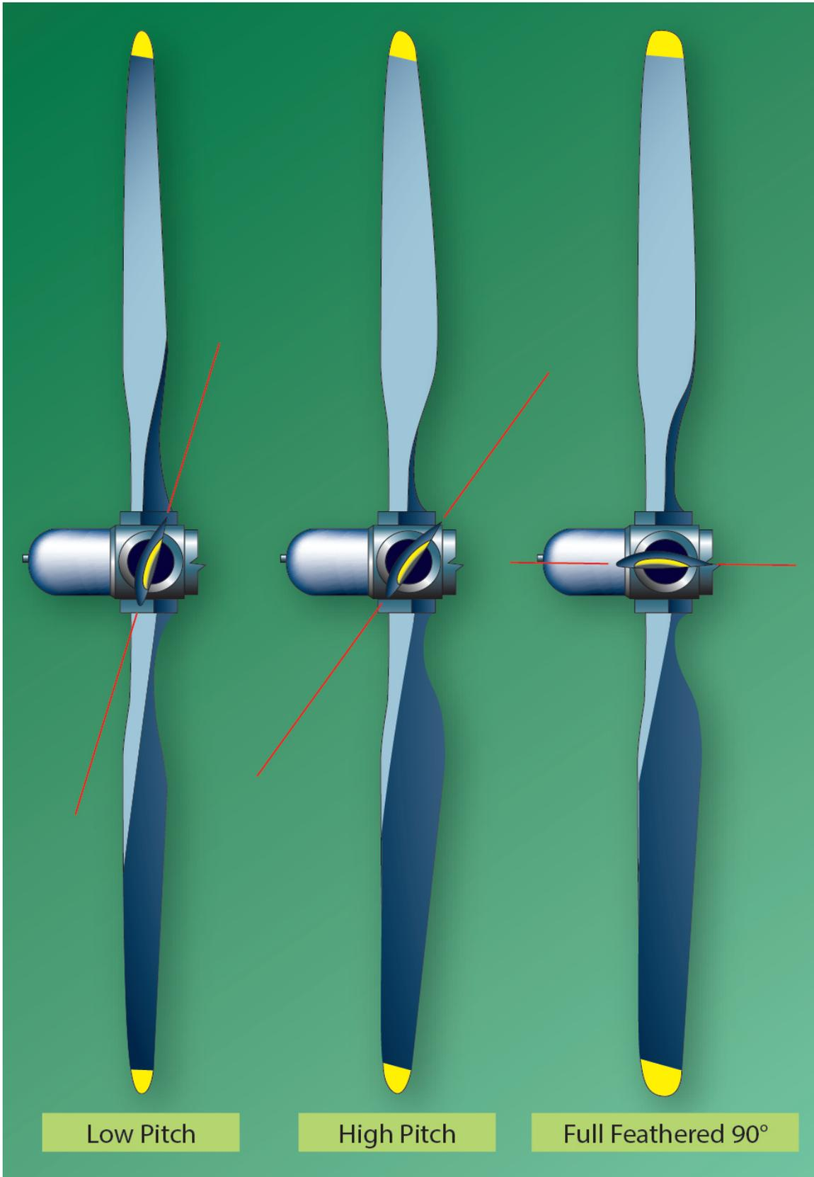
Figure 13-2. Feathered propeller.
