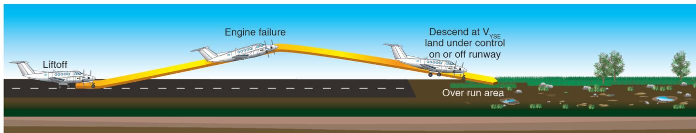
Figure 13-19. Engine failure on takeoff, inadequate climb performance.
