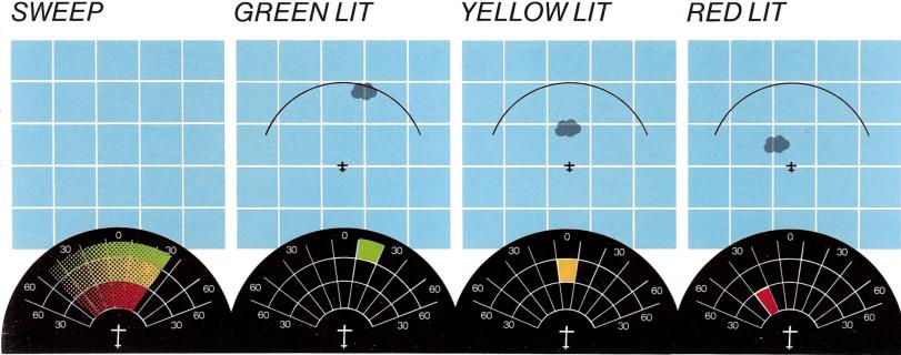
A-1 Example of the test mode. When you push the TST button you will notice that a full color sweep of the total range on the LCD takes place. At the completion of this "sweep," the yellow segment at the 1:30 position will remain lit. (Occasionally the red or green segment may be lit instead of the yellow segment.) When this action is complete, press the CLR button to clear display screen.
