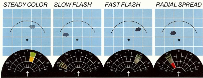
C-1 Steady green and yellow segment at 12:30. Electrical discharges have occurred somewhere between 30 and 100 nm. Deviate course to the left and continue monitoring to watch for thunderstorm development.
