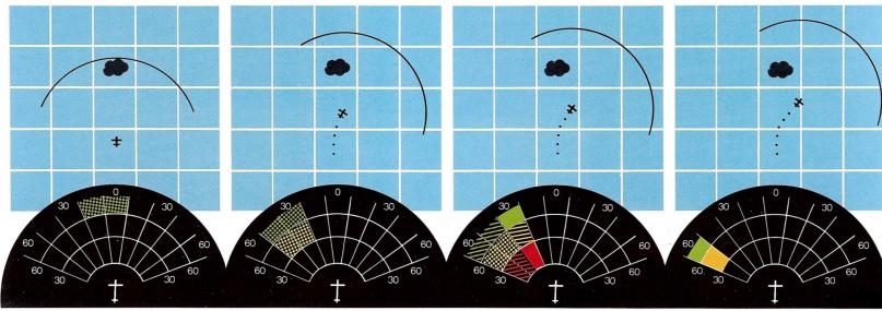
E-1 Severe thunderstorm between 60 and 100 nm straight ahead. Segment is showing fast flashing green indicating a high rate of electrical discharge activity. Course deviation to the right is recommended.
