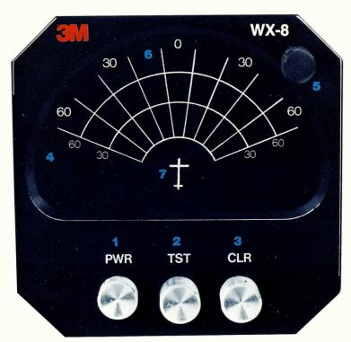
7 Mapping direction indicator. Aircraft diagram indicates position of thunderstorm in relation to aircraft's heading (not necessarily in terms of degrees off compass north or aircraft course).
