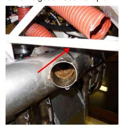
**Arrow Shows Where Interference used to be**
