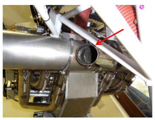
**Arrow Shows Interference of Muffler**
