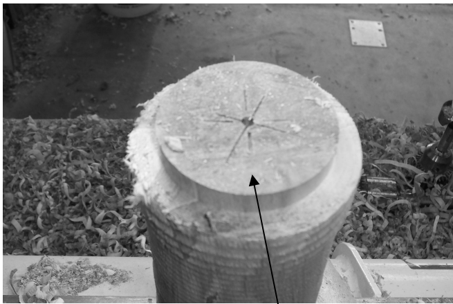
Drill the first hole in the bottom of the body of the pepper mill. This the top of the body where the top was parted off, do not drill here until the body is reversed....
