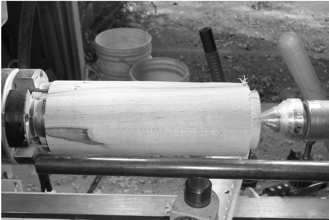
Mount the body of the pepper mill in the chuck (the bottom of the pepper mill should be facing the tail stock)
