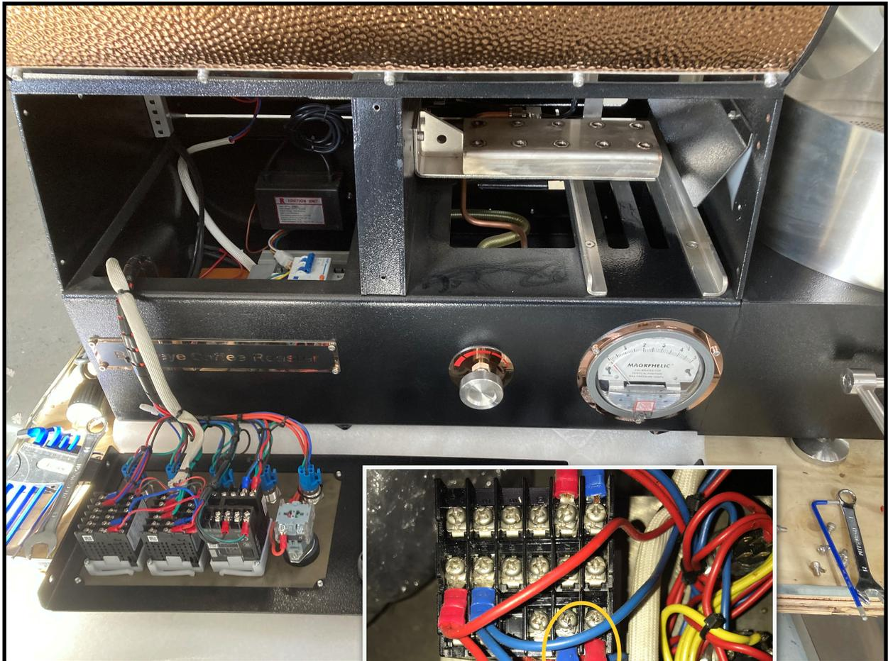
**INSET PICTURE SHOWS WHERE THE TWO WIRES ARE ATTACHED TO EACH OMRON CONTROL.**
