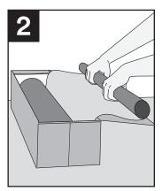
The 3M™ Air and Vapor Barrier 3015NP box can be used as a dispensing unit. Cut the material to the desired length. There are 6" tick marks that can be used for measuring.
