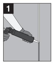
Prepare the wall. Any gaps greater than 1/2" requires backer rod and caulk. Gaps from 1/4"–1/2" require caulk. Concrete walls should have any void areas filled and any fins, mortar joints or screws should be flush with the wall.
