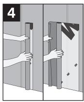
Roll the membrane back against the wall to adhere the starter strip. Unwind the roll against the wall while simultaneously pulling the release liner.
