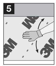
Wipe the membrane down with a feathering motion from the middle outward to obtain a smooth application.
