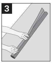
An effective application technique for 3M™ Air and Vapor Barrier 3015NP is to create a starter strip. To do this, crease the release liner approx 1" and peel back to expose the adhesive on the air barrier.
