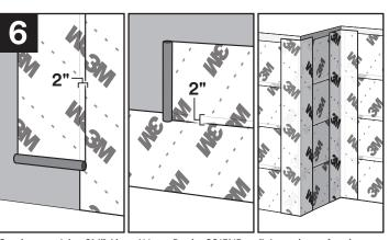
Continue applying 3M™ Air and Vapor Barrier 3015NP until the entire surface is covered, ensuring a minimum of a 2" overlap. Apply in a shingle fashion starting at the bottom of the wall to prevent negative laps. 3M™ Air and Vapor Barrier 3015NP can be applied vertically or horizontally as long as there is a minimum 2" overlap. Inside and outside corners require a minimum 2" wide double layer on each wall.
