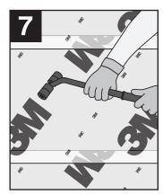
All surface area covered with 3M™ Air and Vapor Barrier 3015NP requires applying pressure with a squeegee or rolling with a J-roller to ensure a tight bond.
