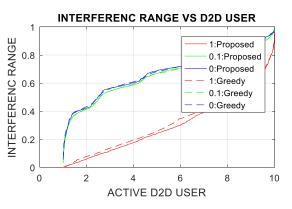
Fig. 7 Interference range vs. active D2D users with LTE users.
