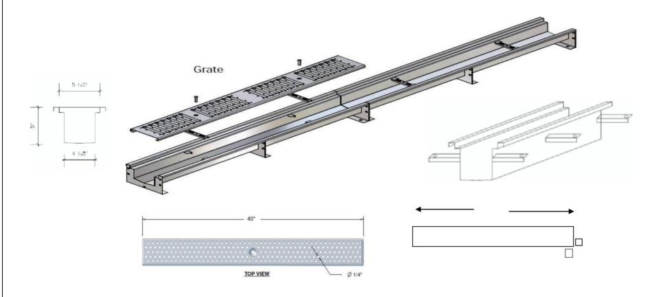
**Engineering Specification:** 6" Wide 14 Ga. 304 Stainless Steel Trench Drain System; Fully Welded End Caps; Outlets; Joints In Factory; Stainless Perforated; ADA; Heel-Proof Class "A" Non-Traffic Grate.
