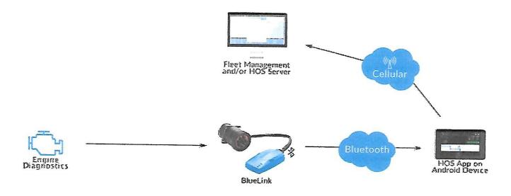
Sends: Odometer, Engine Hour, Engine ON/OFF, VIN #, RPM and Engine Diagnostics Codes
