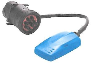
Plug & Play solution, sends engine diagnostics J1939 & J1708 Data to your tablet or smartphone via Bluetooth BLE.
