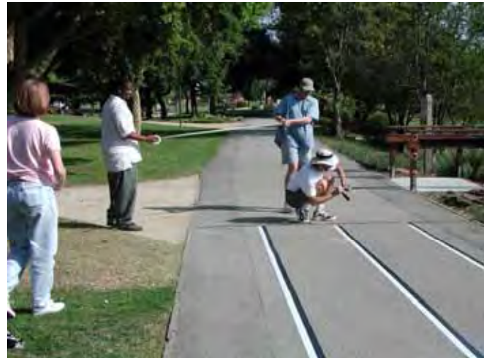
Figure 24. Temporary pavement markings were tested.
