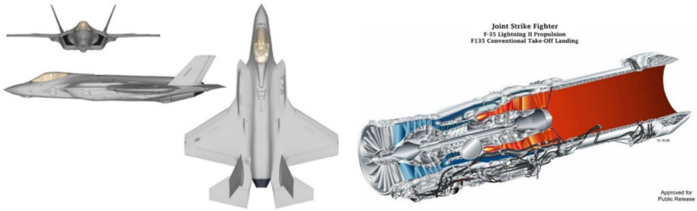
FIGURE VII – THE LOCKHEED MARTIN F-35A CTOL VARIANT 14 AND ITS POWER PLANT PRATT & WHITNEY F135-PW-100 AFTERBURNING TURBOFAN ENGINE. 15
