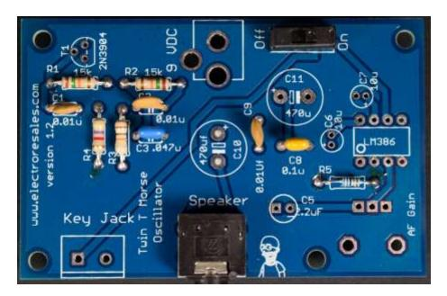
Stage 4 - At this step, add polarized capacitors C5, C6, C7,C10 & C11. Polarity is important here, make sure to align the component with the board markings for '+' or '-'
