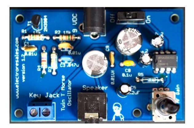
This stage completes the PCB construction, however, before applying power and testing the unit, spend a few minutes checking the position of each part, especially the polarization of the electrolytic capacitors and semiconductors.
