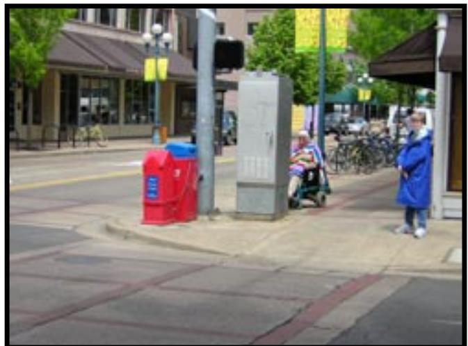
*The signal control box at this corner was identified as being a safety problem because it blocks pedestrians from the view of passing motorists.*
