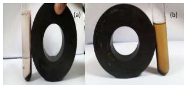
Fig. 1. (a) Synthesized magnetic nanoparticles, and (b) L-asparaginase bound magnetic nanoparticles under magnetic field
