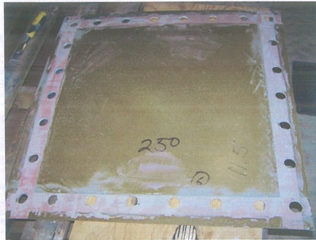
Fig. 9 Panel 6 after drilling and preparation
