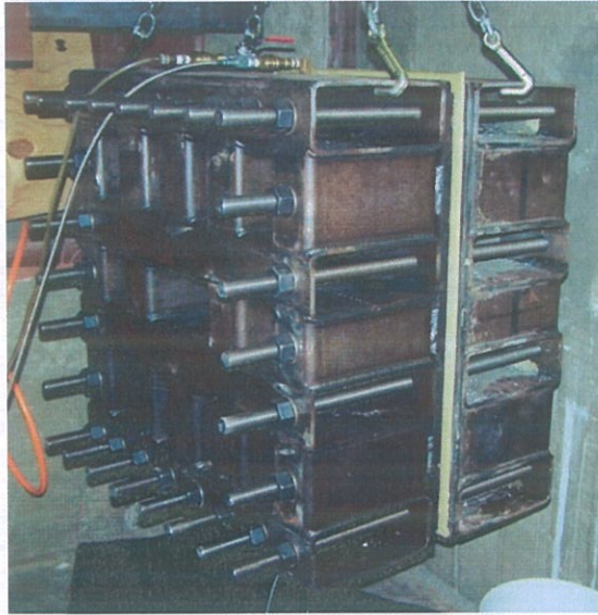
Fig. 6 Assembled Testing Frame with Panel
