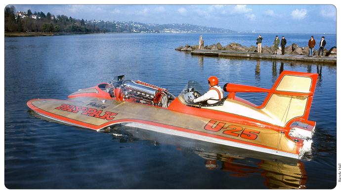
**ABOVE:** Billy Schumacher takes the rebuilt Pride of Pay 'N Pak out for a test drive on Lake Washington before the 1971 season. The boat was reconfigured during the offseason so that the cockpit was moved from the bow to behind the engine. The twin Chrysler Hemis used in 1970 were also replaced with a Rolls-Royce Merlin. RIGHT: The two-time defending champion Miss Budweiser with Dean Chenoweth in the cockpit.
