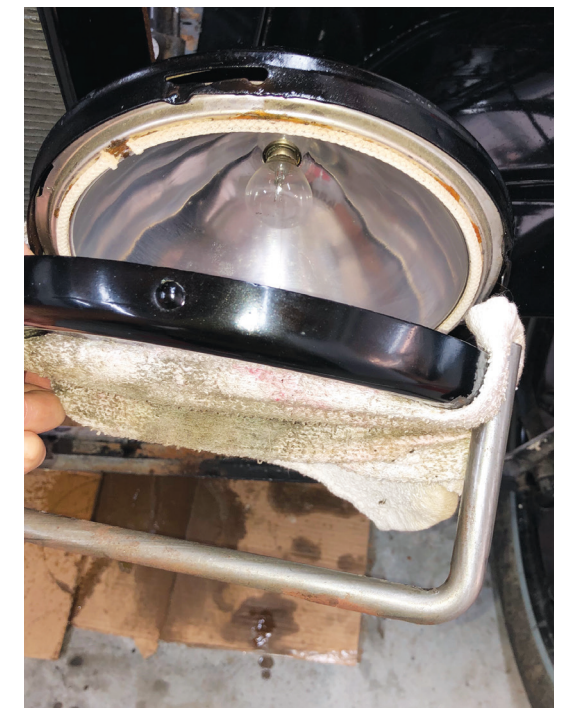
7) Rim and lens are neatly removed, still captured in the rag and tool. (Note: the gap in this reflector cotton cord seal should be at the bottom, for water or moisture to drain away with gravity.)
