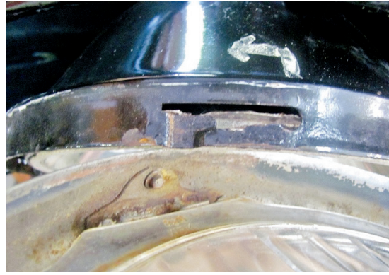
A single rim rivet end shown on lower left. The bayonet groove in the headlight bucket has recess, like a bulb socket, to lock the rim. The left side of the groove has the exit for that rivet.
