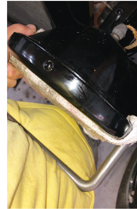
5) Now the rim can be twisted left. Push in hard on the tool to overcome the resistance from the spring behind the reflector. I have found that using my thigh helps to give more power to the push, as both hands are needed to grip the ends of the crossbar tool for the left twist.
