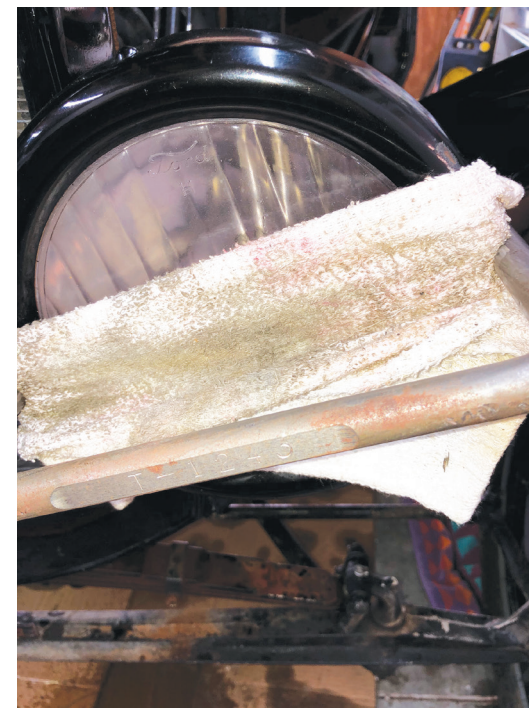
6) After the twist left, the rim and lens are now canted and ready to be pulled away from the bayonet grooves in the headlight bucket.
