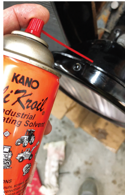
1) Apply your favorite penetrating oil where the surface of the headlight rim meets the headlight bucket. Allow time for the oil to seep in and help loosen any hardened rust or dirt.
