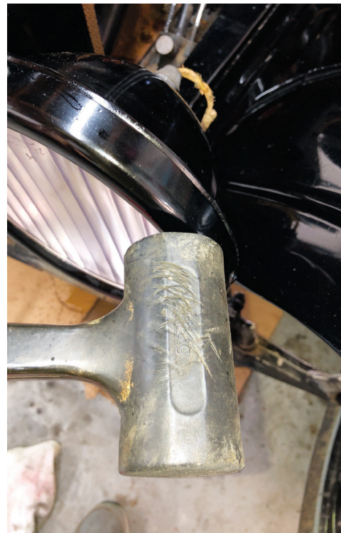
2) Now tap all around the rim with a soft faced dead blow mallet, to free the rim edges that can be stuck to the headlight bucket. You want to see movement all the way around the headlight. Use care and lightly bump the rim. Don't break the lens!
