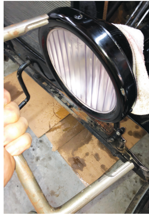
3) With the rim loosened so it can push into the retaining spring behind the reflector, the removal tool is now ready to be used. Note the grooved ends on the tool to mate over two of the rim rivet heads.
