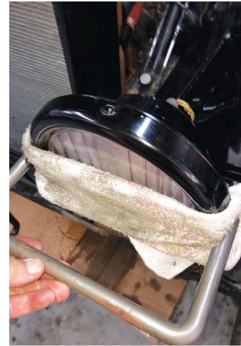
4) Use a rag that is doubled and tucked around the rim. Place it between the tool grooves and the rivet heads to help protect the paint or plating. The rag provides added grip and slip resistance while rotating the rim.
