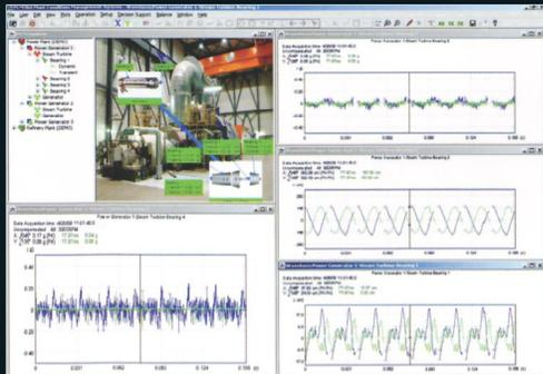
PCM-360 On-line Vibration and Condition Monitoring Software
