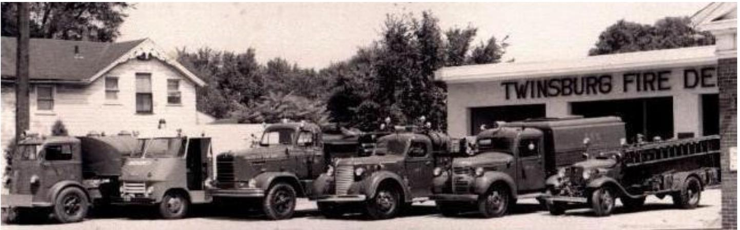
Left to Right: 1942 Autocar tanker with a 3,300 gallon tank, 1958 Chevrolet emergency truck, 1957 FWD 750 GPM pumper with 1000 gallon tank, 1947 Buffalo tanker with a 500 GPM pump and 1000 gallon tank, 1946 Dodge utility truck, and 1934 Ford pumper with 300 gallon water tank. 1934 Ford pump is still owned by Dan Simecek, Fire Chief 1986-1997.
