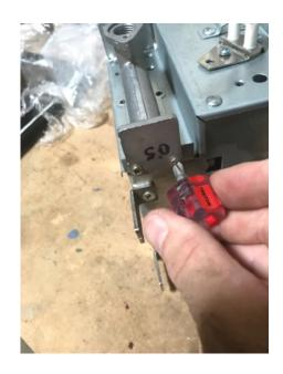
REPLACE WITH NEW INJECTOR ORIFICE TUBE. REATTACH SCREWS. CONNECT GAS LINE USING YELLOW GAS TAPE AND/OR PIPE JOINT COMPOUND TO PREVENT GAS LEAKS
