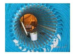
The TDS generator specialist engineers are knowledgeable in the operation of generators and common modes of failure and indications of excessive electromotive forces applied to the electrical winding. These engineers are familiar with the different types of stator high voltage insulation and proper repair procedures for air, hydrogen or water cooled stator bars.
