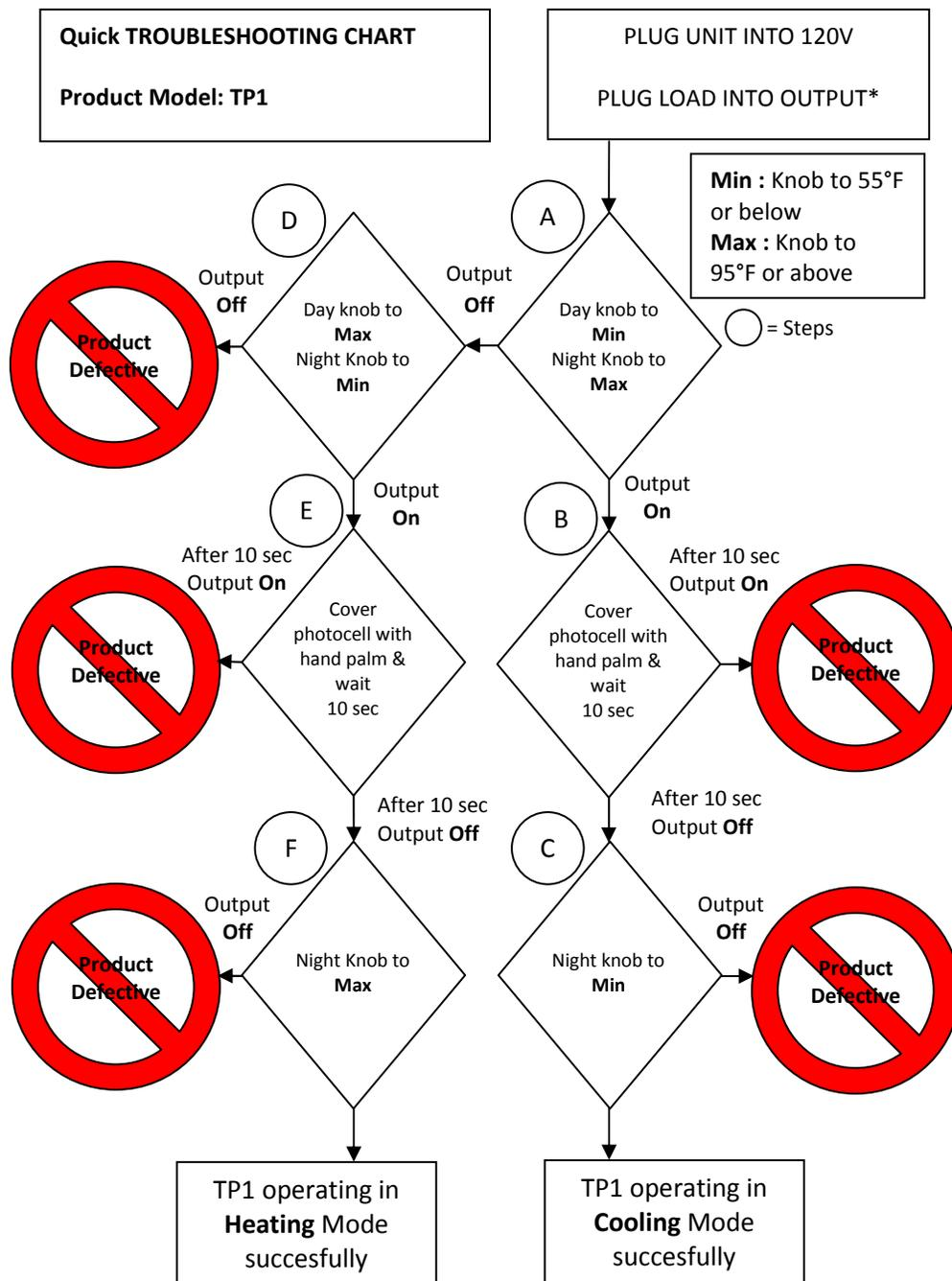
\*Before test, check if load is working properly.
