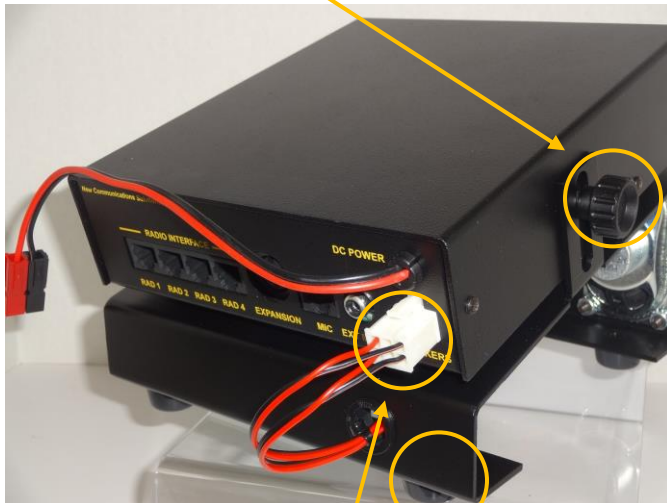
Install Molex connector
