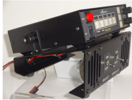
C250 installed with rubber feet
