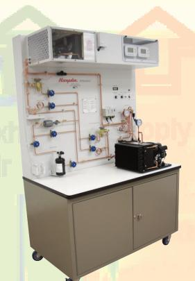
The Hampden Model H-RST-8 Heat Pump Trainer provides students with an introduction to the principal components of heat pump systems.
