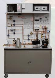
The Hampden Model H-RST-12 Heat Pump Trainer with water cooled condenser provides the student with an introduction to the principle components of heat pump systems.
