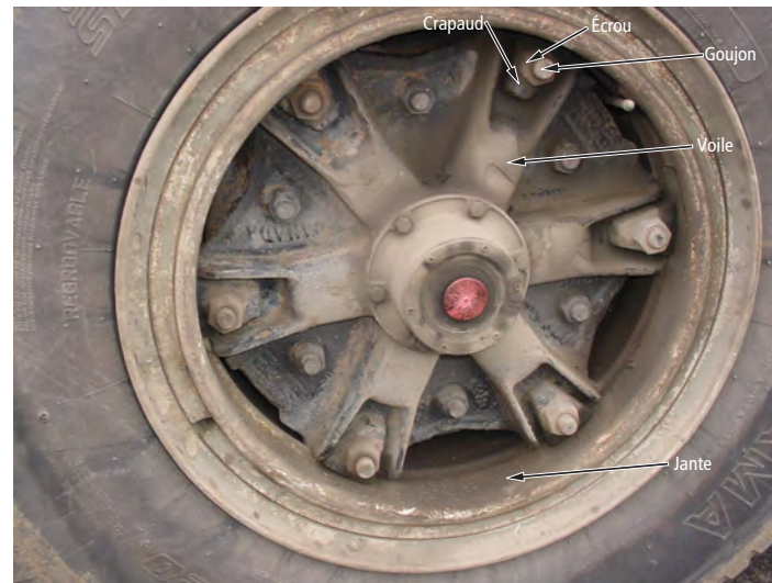
FIGURE 45 | Roue moulée ( spoke wheel )
