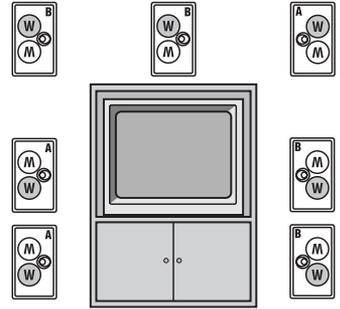
\*Note: When the AMC 800 is used as a center channel speaker and is placed horizontally, the dispersion switch may be set in either position.
