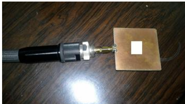
Fig.7. (a), (b) & (c) Fabrication of Prototype DRA using TMM
