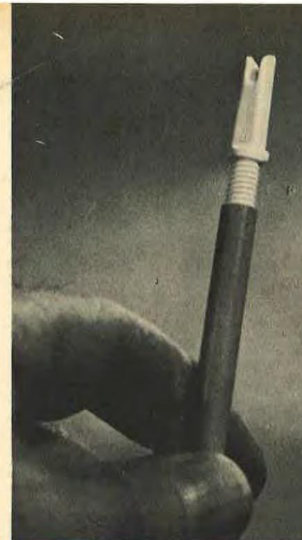
The nylon Nocksert is placed into the tube of the fiberglass shaft, then it is seated to this shaft.
