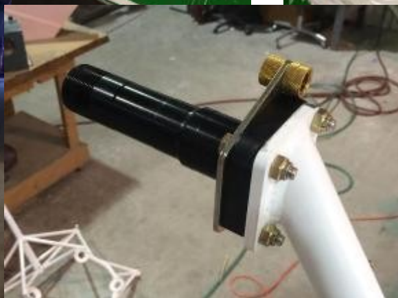
The heavy duty axle for the large engine version of the Lightning.
