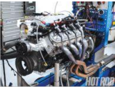
The test motor consisted of a 408 stroker equipped with a forged-steel 4.00-inch stroker c
