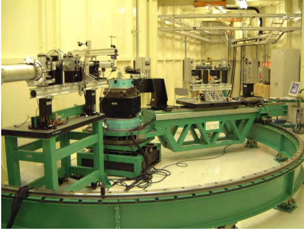
Fig.1: The IXS spectrometer installed in the experimental hutch of BL12XU
