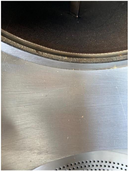
IF YOU CANNOT PUT A 1MM HEX KEY BETWEEN DRUM AND FRONT PLATE YOU SHOULD FOLLOW PROCEDURE IN MANUAL AND ABOVE:
