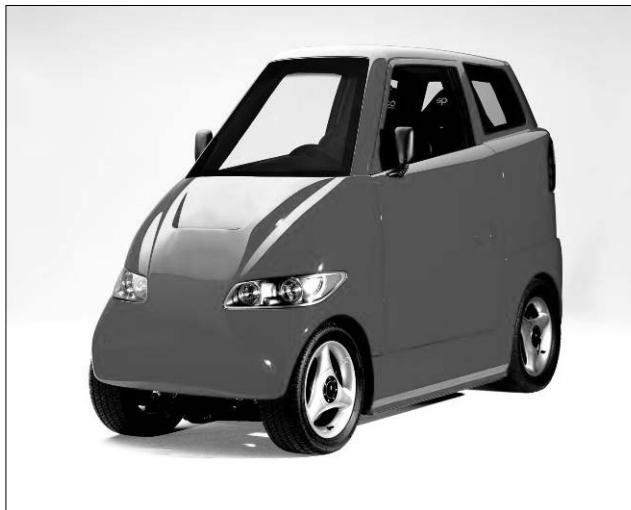
The ultra-narrow Tango T600 is only 39 inches wide, yet claims sports-car handling and a 150 mph top speed.
