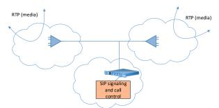
This might occur when there is a central part of the network where the SIP signaling is processed, and a probe could be placed there and listen to all the SIP traffic, but the media don't come to the central location and instead are handled in remotely dispersed gateways. Here the VETap subprobes are used at these remote sites to capture the appropriate media streams under the control of the probe.
