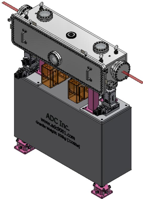
Additionally, the mirror can be positioned within the vacuum chamber through the use of ADC's 300 series precision jacks and slides. This series utilizes NEMA 23 stepper motors with Renishaw encoders to achieve great accuracy and repeatability. These are arranged in a way to provide 5 axis of movement to position the mirror.
