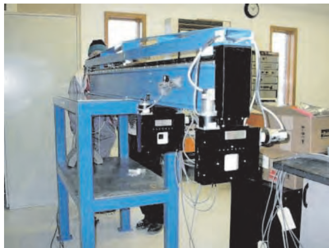
Fig. 1. Incident collimation (prior to installation)
