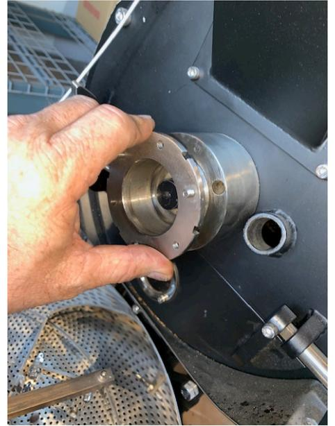
8. Next put bearing into holder. You may need to heat holder to expand so bearing will easily slide into place.
