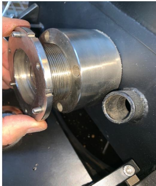
**6.** Once Bearing holder is removed you may need to use a Rod or wood dowel to tap bearing out of holder
