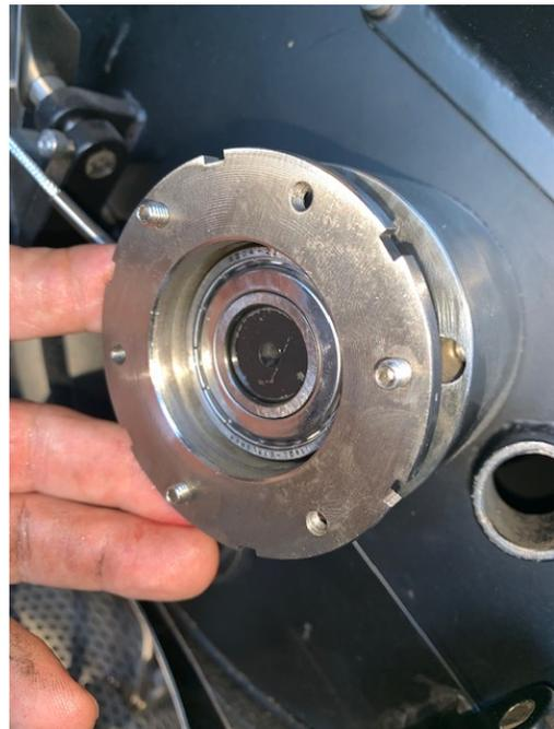
10. Last reassemble and adjust drum to proper distance from front plate and do a heat test
