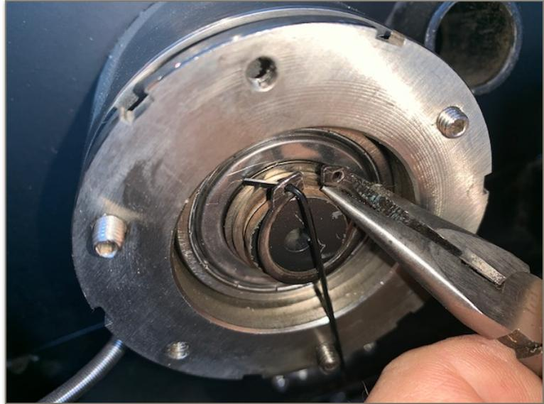
**5.** Next Unscrew bearing holder. If tight you may need gloves or a tool to get it started. If needed lubricate threads.
