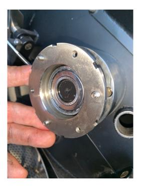
**10.** Last reassemble and adjust drum to proper distance from front plate and do a heat test
