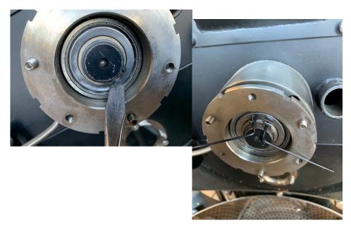
3. Once removed you may find the shaft has a Retaining Clip Ring on it. If so you will need to remove this. You may be able to revoke this with a flathead screwdriver or small needle nose pliers. We found it easy to remove with two 1mm hex keys as shown in image (7) (If your unit does not have the RING CLIP you may proceed to step 5)
