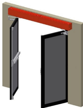
IN/PULL (doors swing under Operators)
