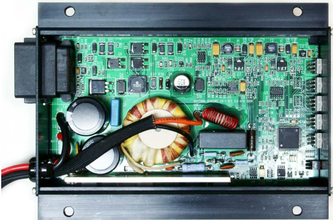
Internal View of Daytona Sensors CD-1
