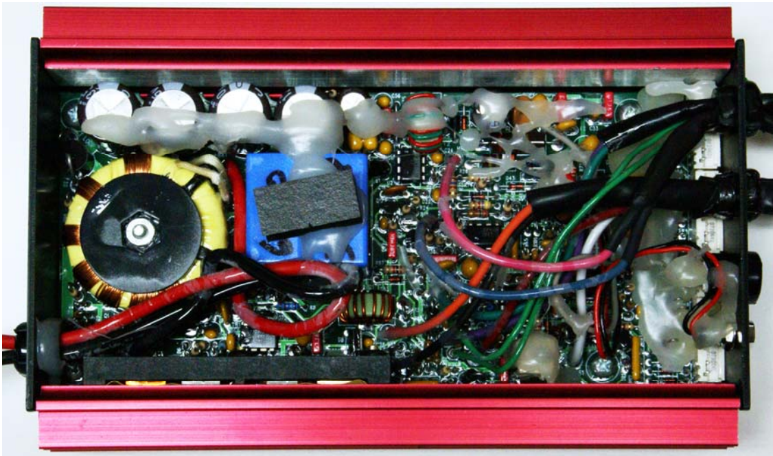
Internal View of MSD Digital 6
