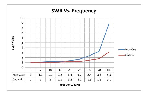
In the next chart which is of resistance change over frequency, it can be seen that the load resistance of the coaxial load decays steadily as frequency increases, while non coax loads show some anomalous changes over 25 MHz these resistance changes illustrate the reasons why a non coax load is a poor choice for higher frequency work. The coaxial load is limited by the resistor composition, and the tendency of certain resistance compositions to exhibit more reactance than others
