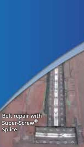
Belt repair with Super-Screw® Splice
