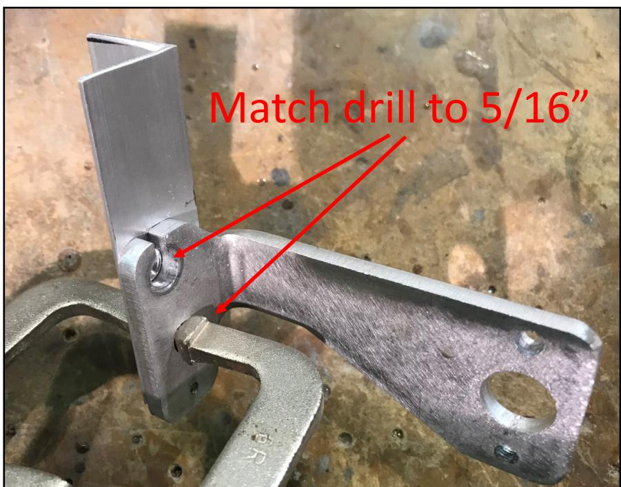
9. The throttle cable hole can now be drilled in the angle
