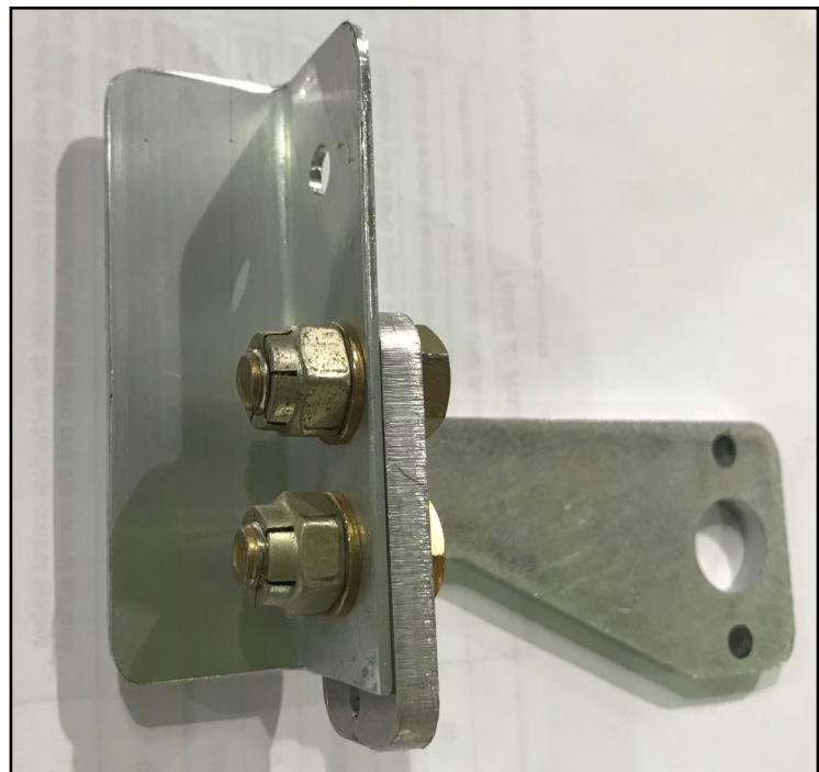
15. Install the assembled throttle bracket we just built with the previously removed gold screws. Use Loctite 242 or similar on the threads.
