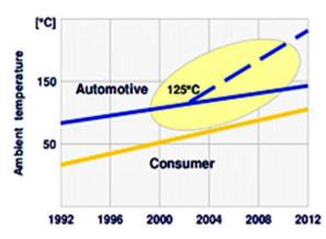
Figure 9 – Increase in operating temperature for the automotive industry [16]
