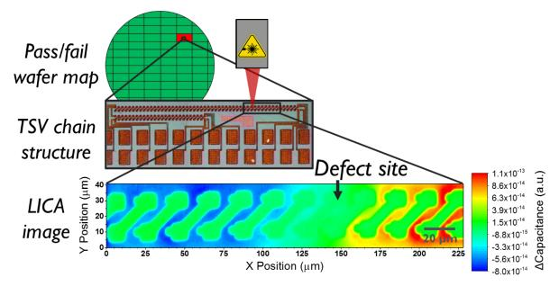
The pass/fail wafer map shows the location of the die failures but contains no information on the exact failure location in the structure. With LICA, failures can be localized more accurately down to a single TSV.
