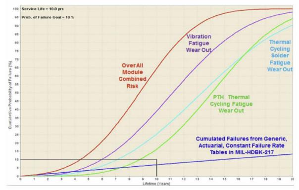
Figure 11 – Physics of Failure Cumulative Failure Risk Life Curves for an Electronic Module [24]
