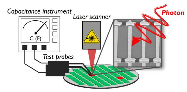
New Technique Localizes Defects in 3D Chips
