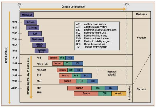
Figure 5 – Past and projected progress in dynamic driving control systems [7, 10]
