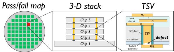
Through-silicon vias are at the heart of 3D chips. TSV failure analysis is indispensable to optimize the production of 3D chips.
