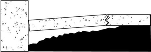
2. Pressure lifts the slab above a cone of "mud" forced through a drilled hole.
