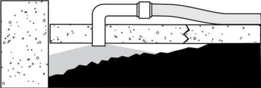
3. Additional holes are drilled to fill voids as needed to support the slab.
