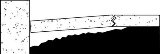
2. Pressure lifts the slab above a cone of "mud" forced through a drilled hole.
