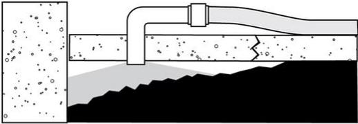
3. Additional holes are drilled to fill voids as needed to support the slab.
