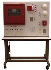
The **Model H-MFA-3C** includes the following: Main Control Panel, Alarm Signal Device, Heat Detector, Smoke Detector, City Circuit Monitor, Pull Station, Remote Annunciator Panel, and Auxiliary Function Panel
