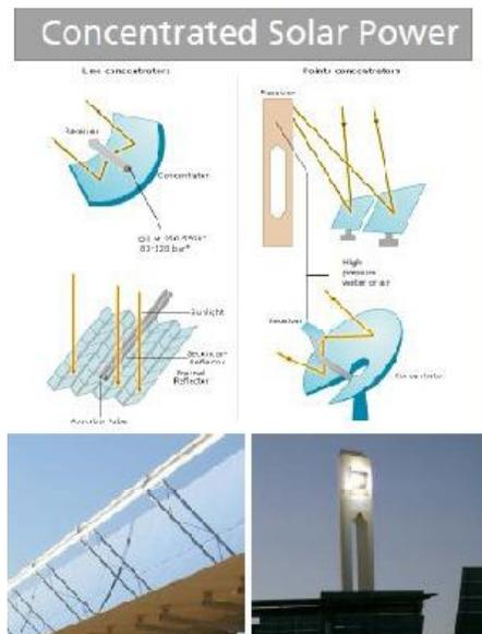
► **CSP technology is based on solar radiation concentration to produce steam or hot air which could then be used on conventional electric plants.**
