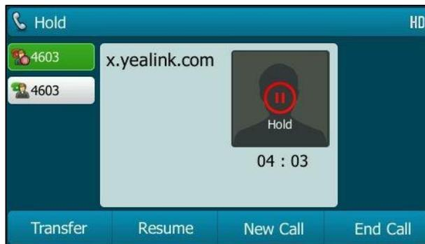
The line key LEDs on phone A slowly flash green and phone B slowly flash red when the shared line call is placed on hold.
