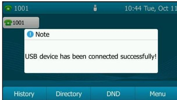
When there is an active call, and you insert a USB flash drive into the USB port on your phone, the LCD screen will prompt "USB device has been connected successfully! Available Recording Time: XX:XX:XX". For more information on the available recording time, refer to [Viewing the Storage Space](#) on page 175.
